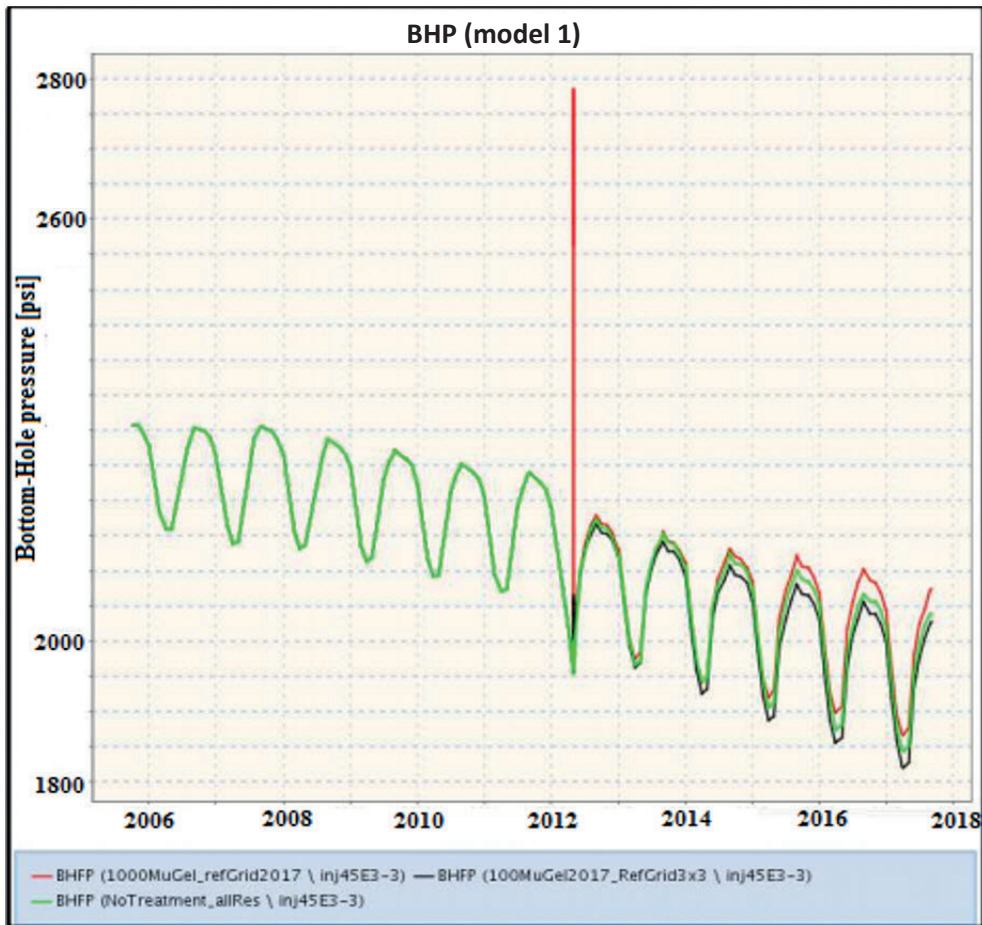
Fig. 9 - Effect of gel injection treatment on bottomhole pressure for reservoir model 1.
