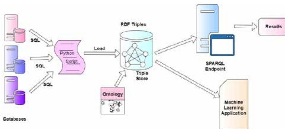
Figure 3: System Architecture
