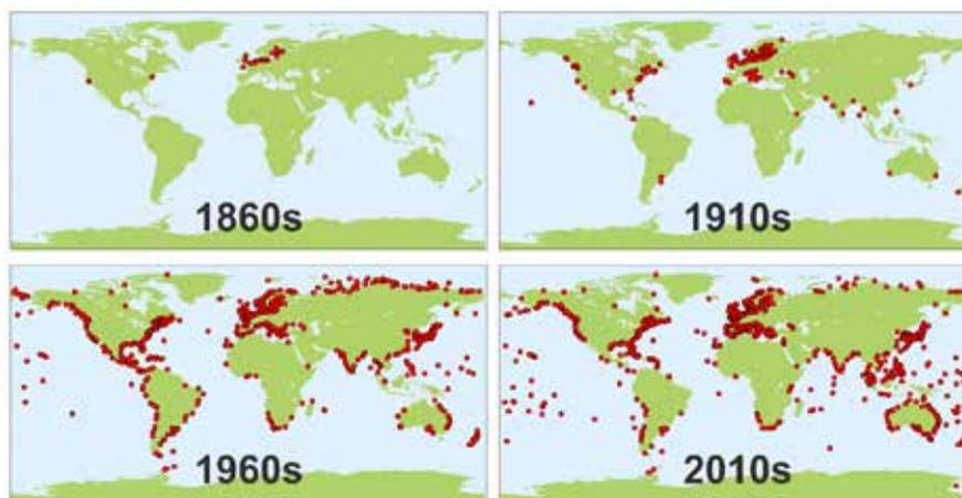
Figure 1: The development of the global tide gauge network over time, as held by PSMSL (<https://psmsl.org>)
