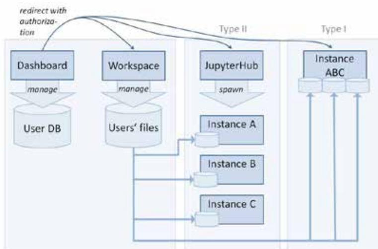
Figure 1: Loosely-coupled structure of VRE services
