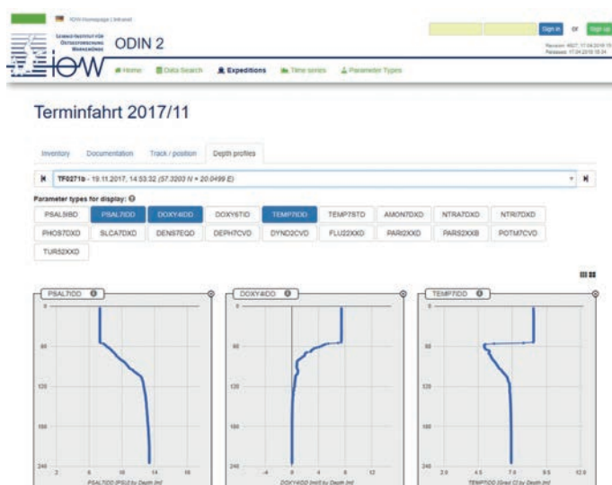
Fig. 2 - Depth profiles available in ODIN2: A single CTD cast at the Gotland Deep in the Baltic Sea, taken November 19, 2017, from surface (top) to 240 m depth (bottom). Profiles from left to right: practical salinity ranging between 7 and 14 PSU, dissolved oxygen concentration (8 to 0 ml/l) and temperature (8 to 4 °C). The stratification of the Baltic Sea is instantly visible.
