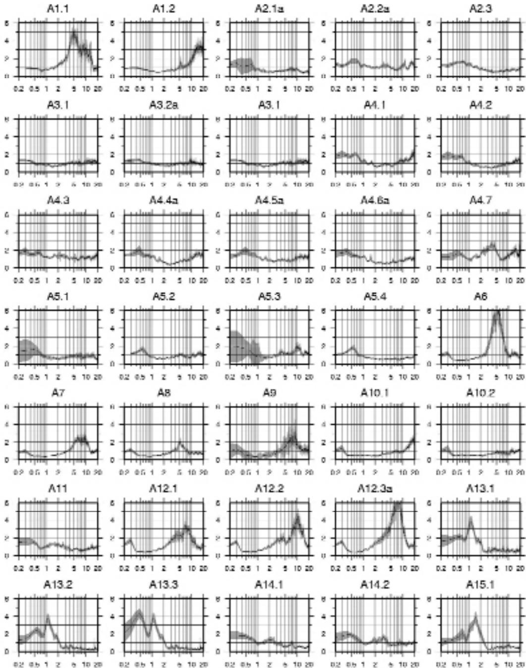
**Fig. 5** - HVSR estimated at all measured sites using the processing of team A. Thick curve: average value. Shaded area: average plus/minus the first standard deviation. Abscissa represents frequency in Hz.
