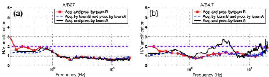
**Fig. 4** - Comparison of HVSR estimated from data acquired independently and simultaneously by team A and B, respectively. Sites are (a) A/B27 and (b) A/B4.7.
