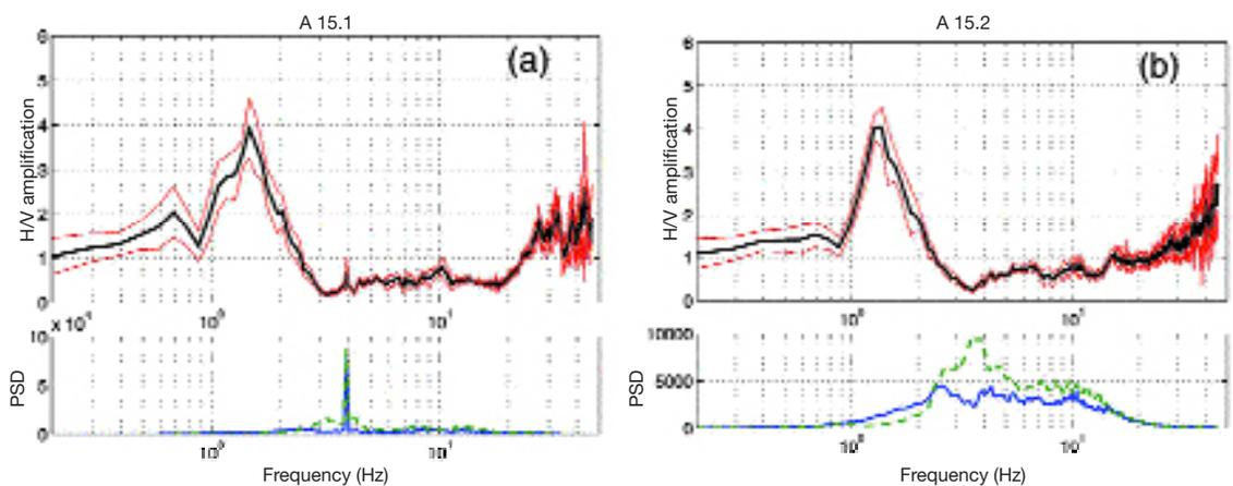
**Fig. 11** - HVSR estimated at the two sites located in the vicinity of the Catania ENEA-ENEL accelerometric station. (a) A15.1, and (b) A15.2. The power spectral density at site A15.2 features a narrow band energy peak at about 4 Hz corresponding to the vibration induced by 400 m - distant factory.
