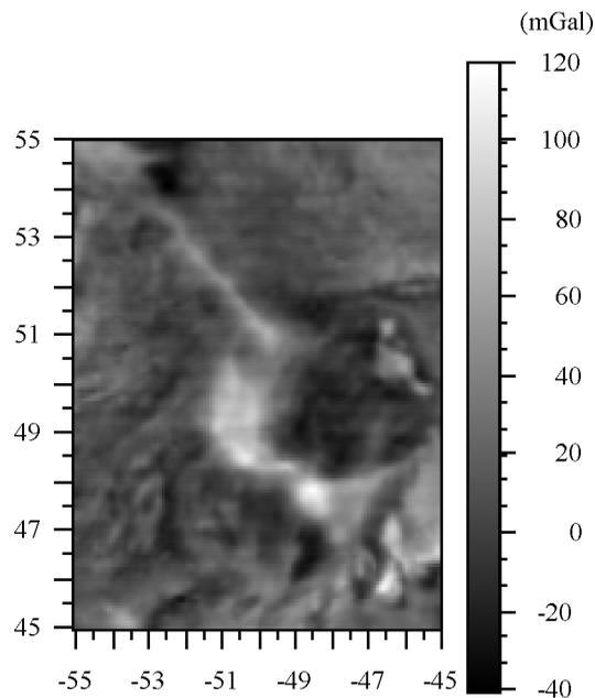
Fig. 2 - Complete gravity anomaly solution by IOST.
