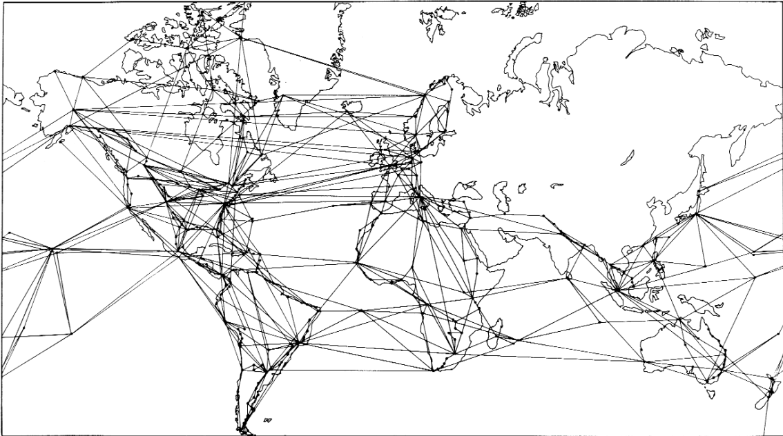
Fig. 3 - The Main Gravimeter connections in IGSN 71.
