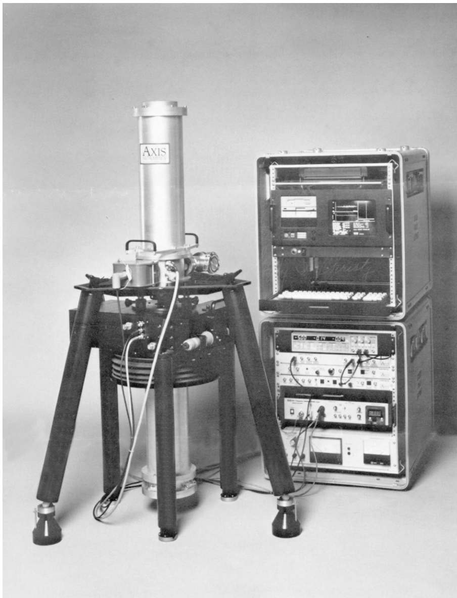
Fig. 6 - The AXIS Instruments Company (now Micro-g Solutions) FG-5 Absolute Gravimeter.
