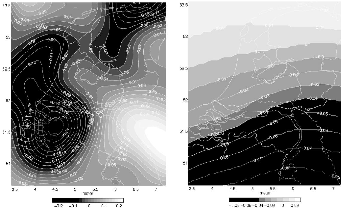
**Fig. 4** - Randomly generated geoid error surfaces based on EGM96 and with Molodenskii weights (left) and with MWG modification (right).
