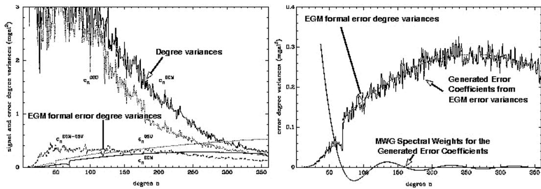
**Fig. 2** - Generation of random error coefficients based on EGM96 including the Meissl/Wong&Gore (MWG) weights (right) based on the formal coefficient error variances (left).
