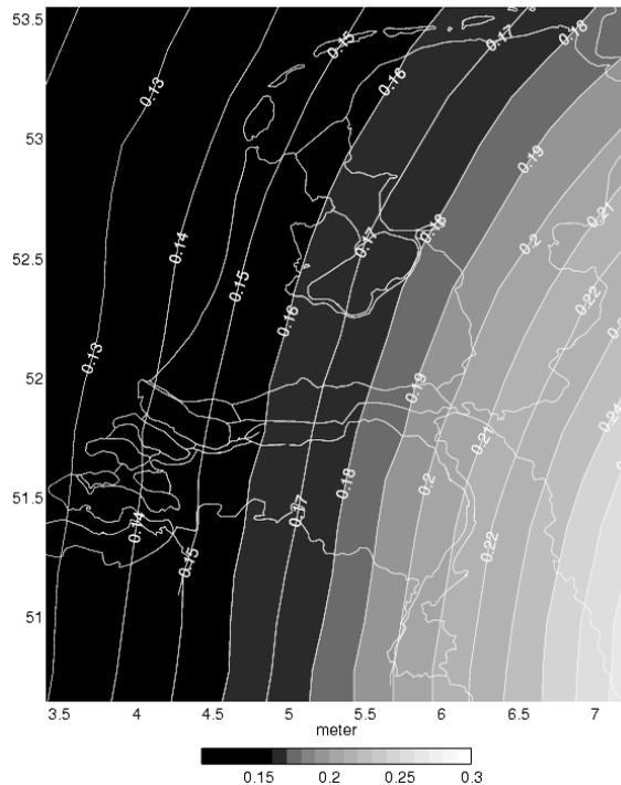
**Fig. 1** - Difference between total gravimetric geoid in the Netherlands based on OSU91 and EGM96.
