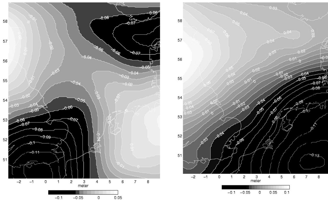
Fig. 3 - Examples of randomly generated geoid error surfaces based on EGM96 and MWG modification.
