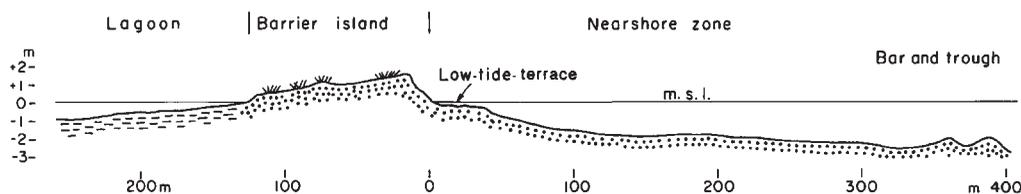
**Fig. 2** - Generalised morphological profile of the new coastal barrier of the Grado Lagoon.
