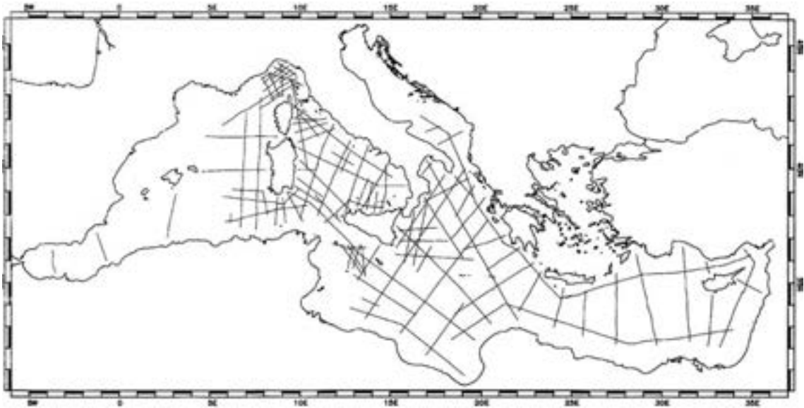
Fig. 4 - The Deep Seismic Reflection Profiles (NVR) in the Mediterranean sea by OGS (MS) and other institutions.
