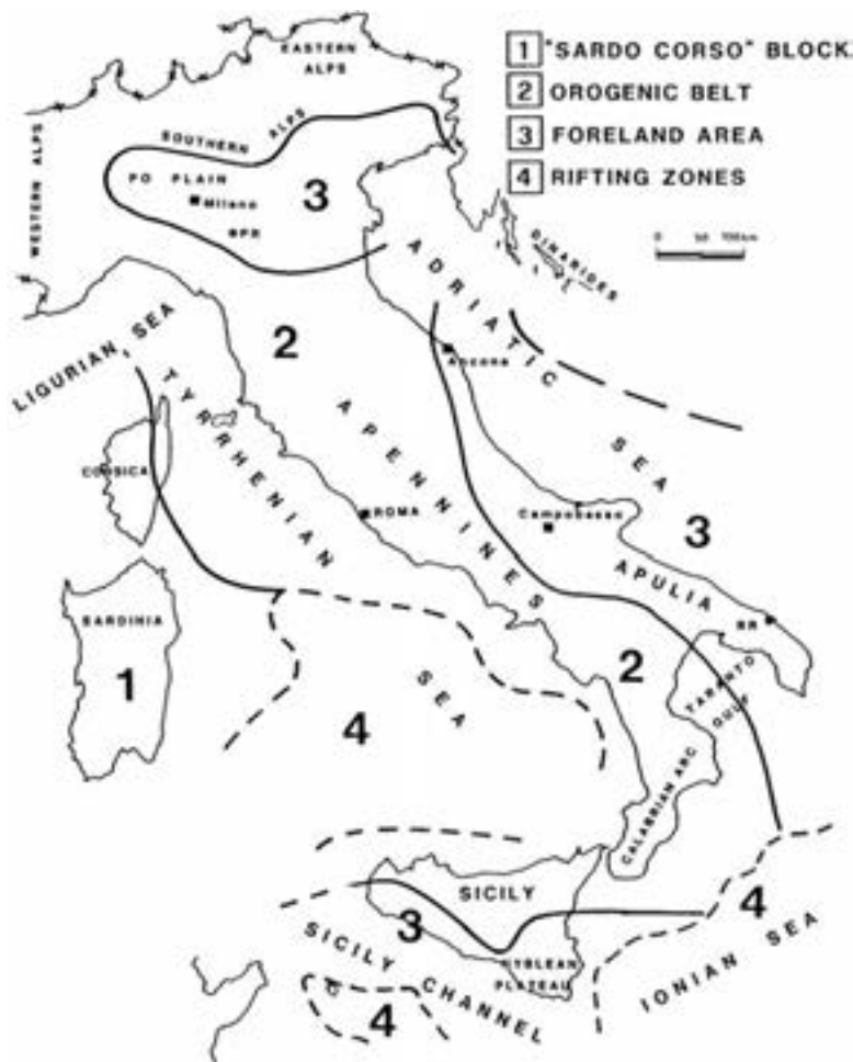
Fig. 12 - The "geomagnetic provinces" of Italy and surrounding seas, evidenced from the aero-magnetic anomalies integrated with other geophysical data (from Arisi Rota and Fichera, 1987).
