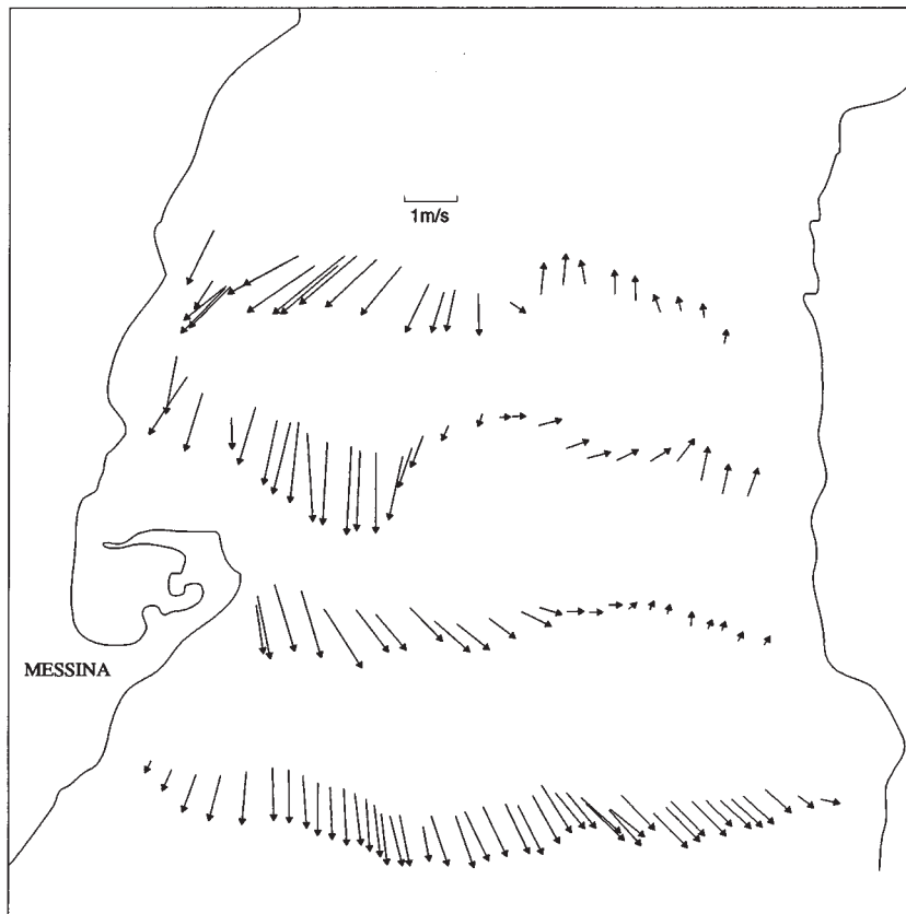
Fig. 2 - An example of the current field at a depth of 8 m found during the low tide phase using an acoustic profiler.
