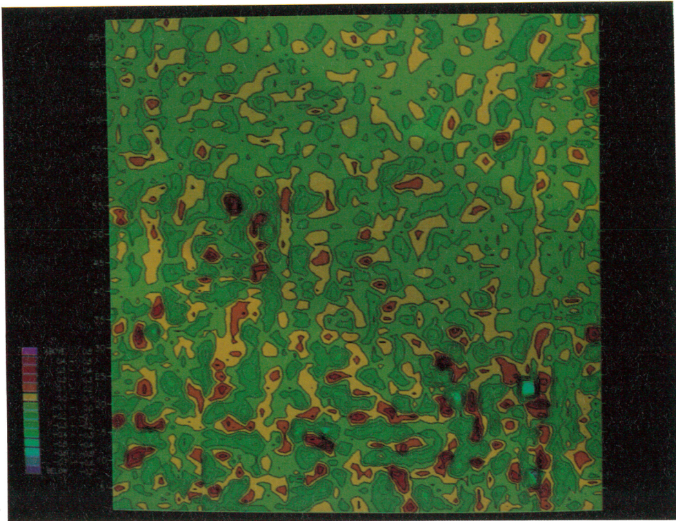
Fig. 8 - 90x90 area. Colour contour map of normalized bidimensional cross-correlation of the data of Fig. 4, using the theoretical anomaly of Fig. 6.
