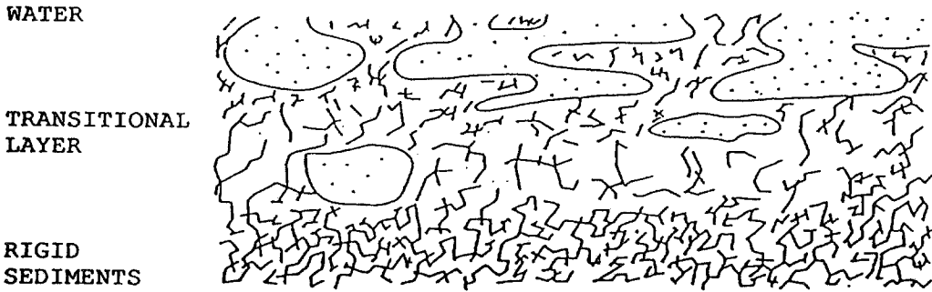
Fig. 2 — Unconsolidated sedimentary layer at the sea bottom in a state close to the rigid-nonrigid phase transition. Hence, there are long-scale variations in rigidity.
